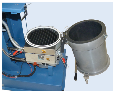
Tiltable tank for easy cleaning and maintenance
