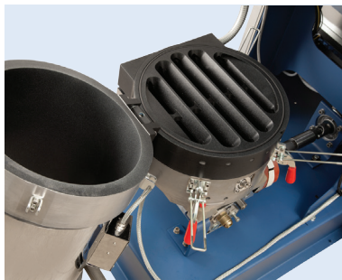
Tiltable tank for easy cleaning and maintenance
